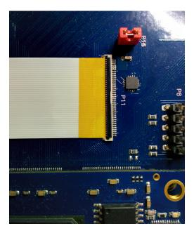
Place the MxxDK Displaykit on MCVEVP without twisting or disconnecting the FPC cable. Mount the MxxDK Displaykit on MCVEVP by using four screws.
