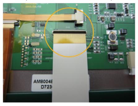
Place the FPC cable in the FPC connector on MCVEVP, the contact side has to be placed towards the TFT PCB so that the isolation of the cable is on top. Close the FPC connector on the MCVEVP carefully.
