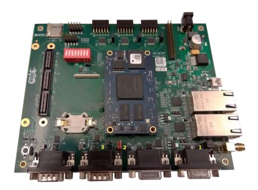
Pin 1 of each header is marked with a yellow dot in the picture.
