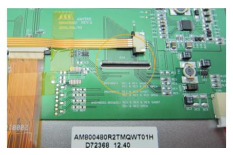
Place the FPC cable in the FPC connector on MxxDK, the contact side has to be placed towards the TFT PCB so that the isolation of the cable is on top. Close the FPC connector on the MxxDK carefully.
