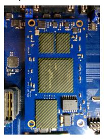
Please make sure that the TOP side of the Altera logo on the CPU is facing the ethernet connector when inserting the SoM into the EVK.
